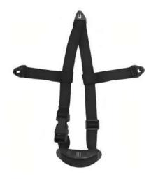
Chin strap in black elastic band 18mm wide and elongation 70-80 with three hooks that attach to the helmet. Due to its design characteristics, it is ideal to be used in the construction industry, shipyards, oil exploitation and mines, construction of tunnels, in sawmills, manufacturing industry, public service companies and in general where there was a risk to losing the helmet.
